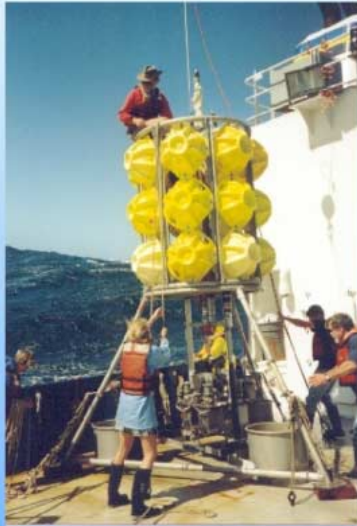
Free-Vehicle Grab Respirometer (K. Smith, SIO)
