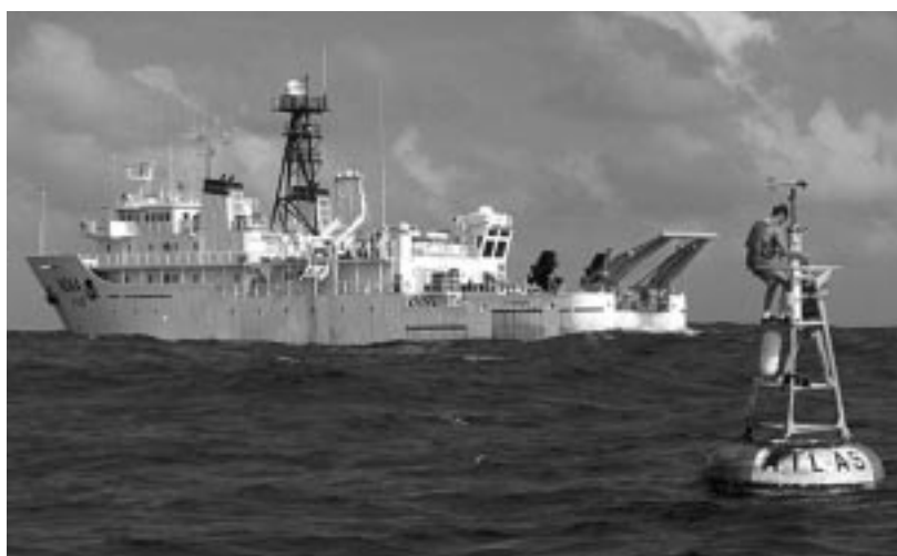
Scientists modify instruments on buoy in equatorial Pacific for real-time transmission of data to laboratories. R/V Ka'imimoana , a NOAA ship, is in the background.
