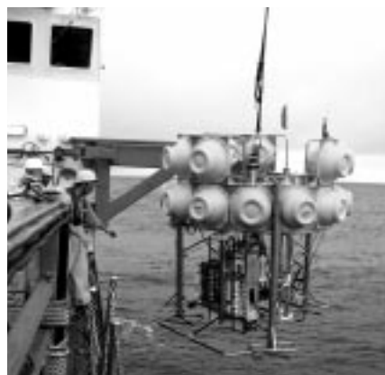
Benthic lander system of the GEOMAR research centre features three benthic chambers equipped with oxygen electrodes and syringe arrays for collecting water samples.
