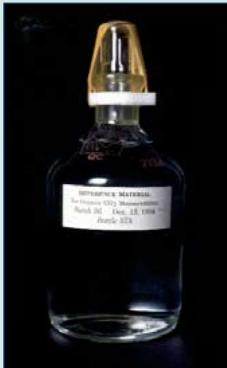
A 500 ml glass bottle containing certified reference material for oceanic CO 2 measurements.
